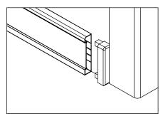
Apply adhesive to the ending parts to secure them in position.
