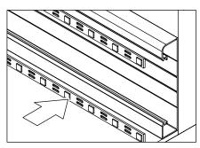
Insert the LED strips into the slots at the top and bottom of the profile.
