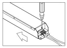
Connect the LED strips and the driver and the driver to the mains. Cables can be carried within the profiles for multi-drive connections. Consult local electricians to obtain accurate results.
