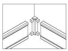
Apply adhesive to the internal corners to secure them in position.
