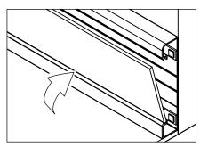
Press the diffuser against the back plate until itclicks into place.
