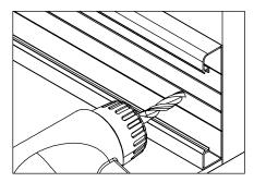
Installation can be done with screws or silicone glue. The correct application must be carefully identified according to the wall material.
