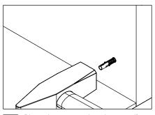
Place the correct dowels according to the wall material into the drilled holes.
