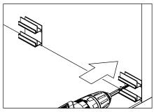
Screw the wall fixation tools to places that are drilled at 50cm intervals.
