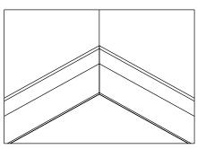
Make sure that the profiles that are cut 45 degrees are fixed to each other completely at the internal corners.
