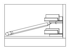
Place the wall fixation tools at 50cm intervals and mark the wall from the screw holes.
