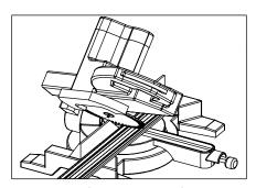
Cut profiles 45 degrees for internal corners.
