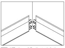
Affix the wall fixation tools in the manner that will be closed to the corners and assemble the profiles that you cut 45 degrees on it.
