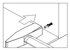
Place the correct dowels according to the wall material into the drilled holes.
