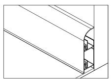
Make sure that the profile nails and the fixation tool's nails are completely connected to each other and be sure that the profile sole is fixed to the floor.
