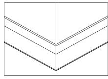
9 Make sure that the profiles that are cut 45 degrees are fixed to each other completely at the external corners.
