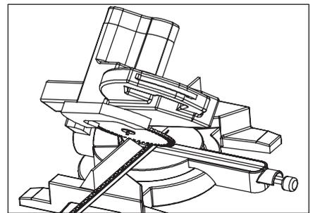
**9** Cut profiles 45 degrees for internal corners.
